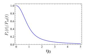
FIG. 2. Probability  $P_e(t)$  of exciting a two-level system in a spherically symmetric trap and its dependence on the effective Lamb-Dicke parameter  $\eta_0$  [see Eq. (5.7)]: the center-of-mass state  $\hat{\rho}_T(\tau)$  is assumed to be an isotropic Gaussian state. The spontaneous decay rate is assumed to be large compared to the trap frequency, i.e.,  $\Gamma \gg \omega_{\text{trap}}$ .
