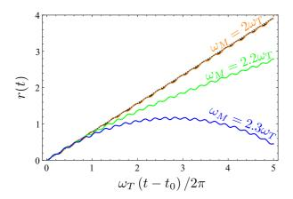
FIG. 4. Time evolution of the squeezing parameter r(t) for  $\delta = 0.5$ : numerically exact results for modulation frequencies  $\omega_M = 2\omega_T$  (orange solid line),  $\omega_M = 2.2\omega_T$  (green solid line),  $\omega_M = 2.3\omega_T$  (blue solid line), and the associated approximation (dotted line).
