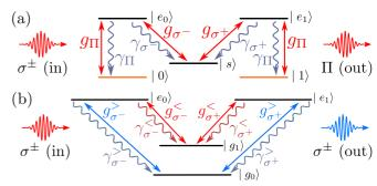
FIG. 5. Atomic level structure for converting a polarization encoded photonic qubit encoded into a matter qubit (a) and for converting the frequency of a polarization encoded photonic qubit (b).
