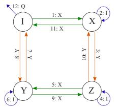
FIG. 4. (Color online) A Eulerian path for a dynamically corrected gate operation Q.
