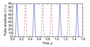
FIG. 2. (Color online) The pulse sequence used to implement the iSWAP gate. This figure shows the pulse sequence used for both of the gate qubits, where solid blue signifies a pulse in the X direction and dashed red signifies a pulse in the Y direction. Neighboring qubits use the same pulse sequence, but with X and Y swapped if their coupling is to be eliminated.
