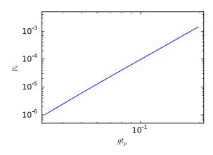
FIG. 6. (Color online) The probability of error  $p_e$  for the singlequbit  $R_x(\pi/2)$  gate depending on the pulse width  $t_p$  in double logarithmic scales. The dependency is read out to be approximately  $p_e \sim (gt_p)^4$ .
