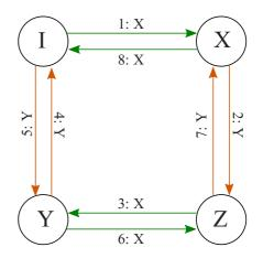
FIG. 1. (Color online) A Eulerian path decoupling sequence for a single qubit. I, X, Y, Z correspond to the Pauli operators  $1, \sigma_1, \sigma_2$ , and  $\sigma_3$ . The vertices represent the decoupling operators  $g_j$ ; the directed edges denote the transitions between the  $g_j$  due to the decoupling pulses  $p_j$ .
