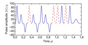
FIG. 5. (Color online) The pulse sequence applied to a single qubit to implement a dynamically corrected  $R_x(\pi/2)$  gate with Gaussian pulse shapes. Solid blue indicates that the pulse generator is acting along the X axis; dashed red indicates a pulse along the Y axis.
