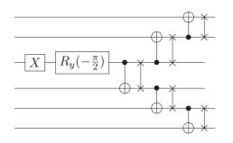
FIG. 8. A quantum circuit to entangle all qubits in a quantum register in a GHZ state. In this figure, the CNS gates are represented by a directed CNOT gate followed by a SWAP gate.
