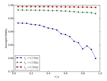
FIG. 9. (Color online) Averaged fidelity for a GHZ state achievable on a four-qubit chain for different values of the pulse duration  $t_p$  (Gaussian pulse shapes were used), when the qubit eigenenergies differ from each other. The  $\Delta_i$  are randomly sampled from a Gaussian distribution with standard deviation  $\sigma$ . The plotted results were averaged over 100 runs.
