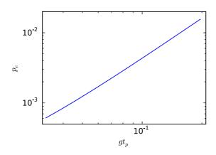
FIG. 3. (Color online) The probability of error  $p_e$  for the iSWAP gate depending on the pulse width  $t_p$  in double logarithmic scales. The dependency is read out to be approximately  $p_e \sim (gt_p)^{1.8}$ .
