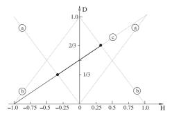
**Fig. 2.** Six-state protocol: region of the parameters D(QBER) and H for which the two-qubit state  $\tilde{\rho}_{AB}^{(j_1)}$  is separable (thick solid line). The various constraints that these parameters satisfy are indicated by straight dotted lines. Specifically, (a) equation (20); (b) equation (19); (c) equations (16) and (28). The protocol operates along the solid lines.
