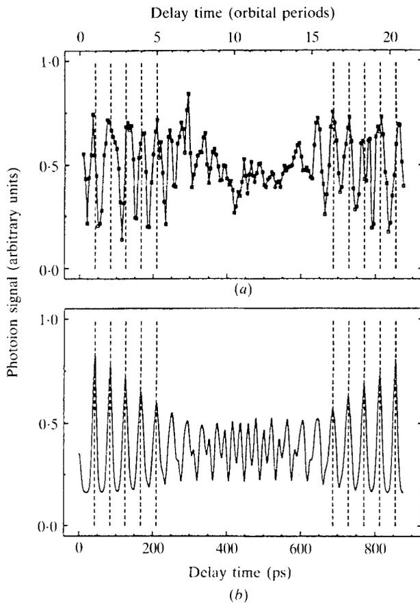
**Figure 3.** The photoionization signal as a function of the delay between the pump and probe pulse time shows the evolution of the radial wave packet: (a) experiment and (b) theory (reproduced from ten Wolde *et al.* (1988) with the authors' permission).
