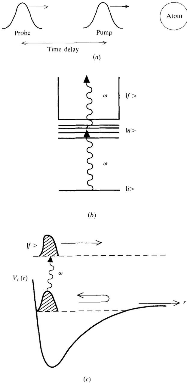
**Figure 2.** Pump-probe scheme to excite and detect the motion of a radial Rydberg wave packet. (a) Time-delayed pump and probe beams exciting the atom (b) Atomic excitation scheme: the first (pump) pulse excites the wave packet which is probed by the second time-delayed pulse (c) The return of the wave packet to the ion core is probed by the second pulse which ionizes the electron near its inner classical turning point.
