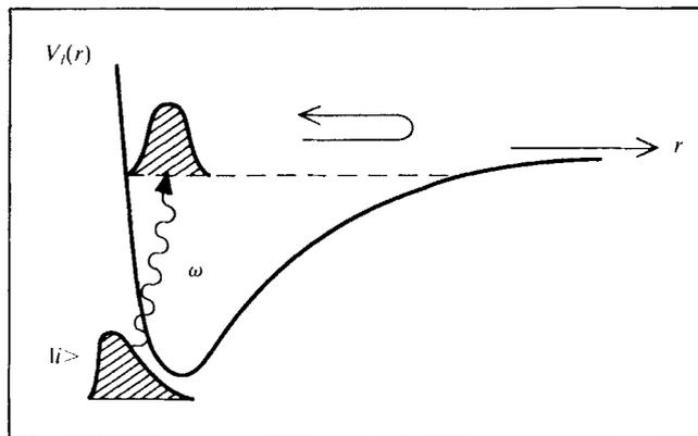
**Figure 1.** Excitation of a radial Rydberg wave packet by a short laser pulse. Initially the electron is in the ground state  $|i\rangle$ . A short laser pulse excites a superposition of Rydberg states. This corresponds to a wave packet moving in the effective radial atomic potential (given by the Coulomb potential and the centrifugal barrier).
