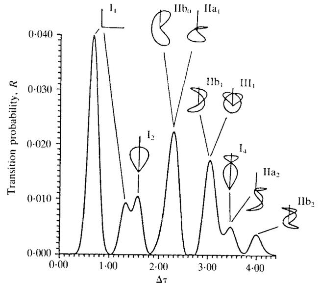
**Figure 4.** Rydberg atom in magnetic field: the transition probability for a Raman process as a function of the time delay between the two laser pulses. The peaks are associated with closed orbits where the wave packet returns to the ion core. The magnetic field is  $B = 0.47$  T. Time is measured in units of the Larmour precession time  $T = 76$  ps.
