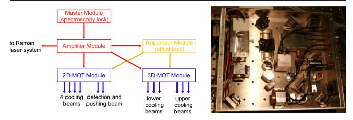
Fig. 7 Left: scheme of the modular laser system; right: a picture of the master laser module
