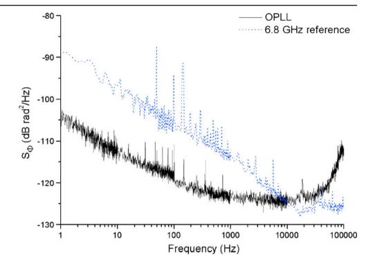
noise is among the lowest levels ever reached (Cheinet et al. 2008). The achieved locking bandwidth is slightly above 4 MHz. If this OPLL phase noise was the main contributing factor to overall accelerometer sensitivity, a single-shot sensitivity  $\delta a/a$  of  $2 \times 10^{-10}$  would be achieved.
