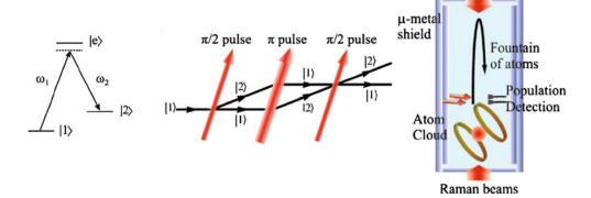
**Fig. 1** Atom interferometry accelerometer; from *left to right*: Raman transition between the hyperfine levels of an alkali atom; Mach–Zender atom interferometry scheme implemented with three Raman pulses  $(\pi/2 - \pi - \pi/2)$ : the direction of the *red arrows* represent the effective momentum transferred in the stim-
