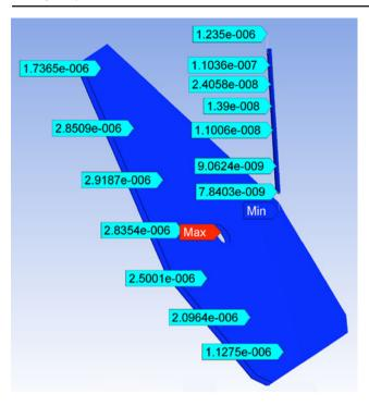
**Fig. 5** Numerical calculation of residual magnetic field inside the capsule; the *labels* indicate the amplitude of magnetic field (in Tesla) on different points of the diagonal  $\mu$ -metal plane and along the atomic trajectory (from the *center* of the chamber to the *upper edge* of the tube) when an external bias field of 50  $\mu$ T is applied along the vertical axis
