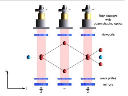
**Figure 4.** Interferometer scheme in a time series. The sequentially applied laser pulses split, reflect, and recombine the atomic wave-functions. The color of the balls represent the two hyperfine levels of the rubidium atoms. After release, the atoms are in the excited state (red balls), and during the atom interferometry sequence in the ground state (red circles). In this sketch perfect beam-splitting efficiency is assumed.
