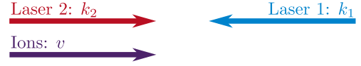
FIG. 2. Two counterpropagating lasers with wave number vectors \mathbf{k}_1 = -k_1\mathbf{e}_z and \mathbf{k}_2 = k_2\mathbf{e}_z interact with the ions, which move with velocity \mathbf{v} = v\mathbf{e}_z parallel to laser 2. Wave numbers and scalar velocities are positive quantities k_i, v > 0 .
