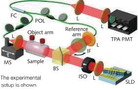
for the ghost spectroscopy signals as a function of the refdemonstration using erence frequency. It is thought a superluminescent that ghost spectroscopy had laser diode source. not been achieved using a thermal light source because
