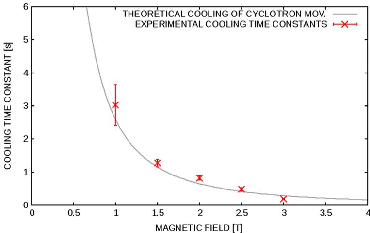
**Fig. 3** The measured cooling time constants (red) in comparison with the theoretical prediction for different magnetic fields (grey). One should note that, aside from the good general agreement, the remaining deviations between experiment and theory arise from experimental parameters like field inhomogeneities and particle-particle interactions, and are not expected to vanish in the experiment [19]
