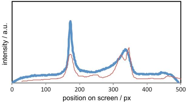
**Fig. 2** Ion deceleration in the RFQ as seen by the energy analyser. The thin, red line is the reference signal from the offline tests and the thick, blue line is the online signal achieved at HITRAP. The low energy part, i.e. the decelerated ions' signal is the peak to the left. The peak to the right is the undecelerated part of the beam
