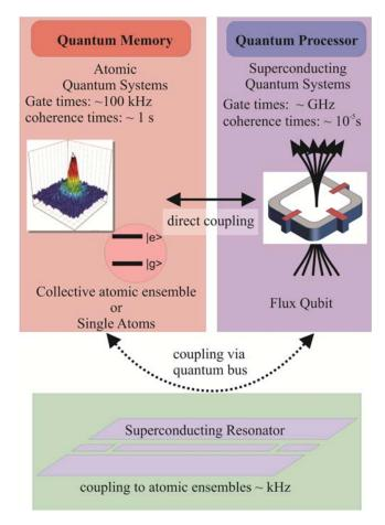
**Figure 11.** Vision of a hybrid quantum device: quantum states are processed in a superconducting circuit and stored in an atomic ensemble. The coupling is mediated either directly or via a quantum bus.
