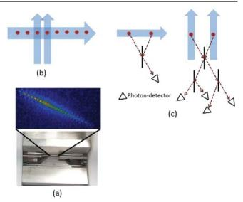
**Figure 6.** Schematic of quantum information processing (QIP) using trapped ions: (a) a linear ion trap with blade structure and a large ion crystal that forms the hardware for both quantum computation (b) and communication (c). Two ion gates are operated by using individual addressing as in (b) for computation. The heralded communication scheme in (c) can be made deterministic by having a cavity around each ion trap.
