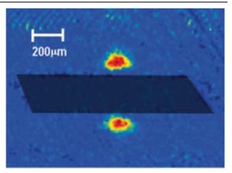
**Figure 10.** Atoms levitating in a magnetic field generated by a distinct vortex pattern in a superconducting square (indicated by dark blue area). The lower cloud is a reflection of the atomic cloud from the surface.
