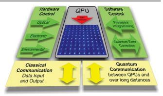
**Figure 9.** Block diagram of a neutral atom quantum processing unit (QPU), consisting of a 'qubit RAM', expected to contain on the order of 10 000 qubits, embedded in the required control and communication periphery.
