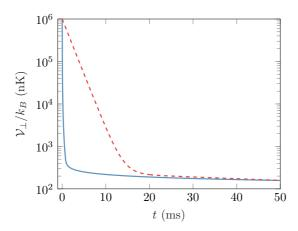
FIG. 3. Potential depth  $V_{\perp}(t)$  versus time t. The red dashed line shows the ramp resulting from the biexponential ansatz, whereas the blue solid line is the optimal adiabatic ramp.
