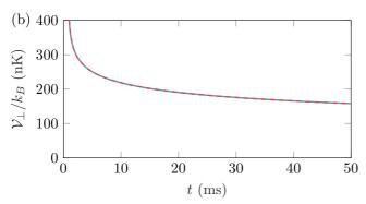
FIG. 6. Optimal adiabatic potential ramp  $V_{\perp}(t)$  versus time t: comparison between the numerical solution of the Euler-Lagrange equation (blue solid lines) and the analytic approximation (dashed red lines) given in Eqs. (60) and (62). For t < 0.7 ms (a) interband excitations dominate, whereas for t > 1 ms (b) intraband excitations are the most relevant.
