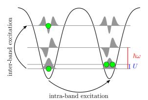
FIG. 1. Excitation pathways in a microtrap array: interband excitations dominate in deep traps since intraband tunneling is exponentially suppressed. However, for shallower potentials, intraband tunneling prevails as long as the two-particle interaction energy  $U \equiv U_{iii}^{0000}$  remains smaller than the band gap  $\hbar\omega$ .
