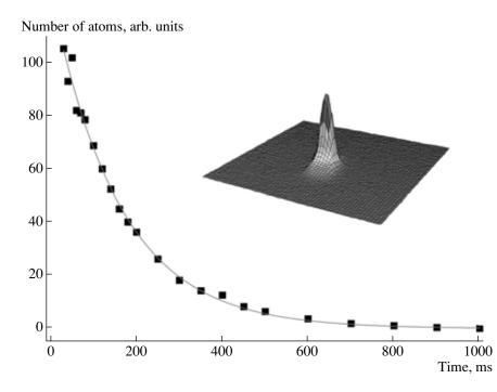
**Fig. 2.** Number of atoms remaining in dipole trap as a function of time. An exponential fit to the data yields a storage time of 166 ms. Inset: Density distribution of atoms in a single dipole trap obtained by using a single microlens in the setup depicted in Fig. 1.
