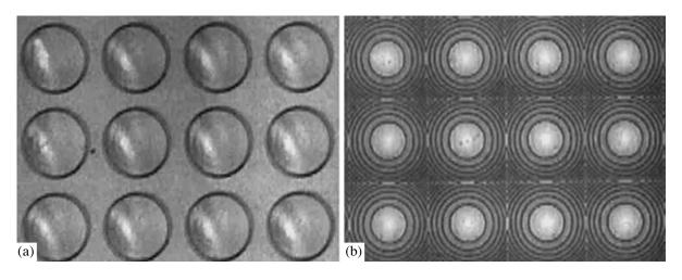
Fig. 3. (a) Refractive and (b) diffractive array of spherical microlenses.
