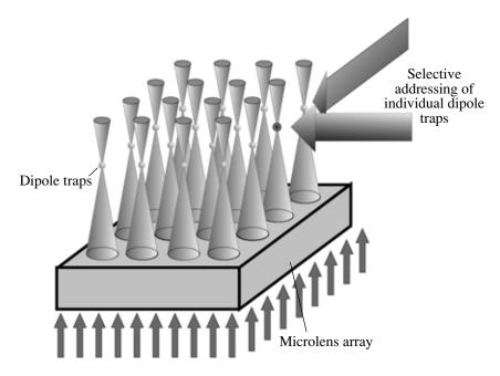
Fig. 4. Two-dimensional array of dipole traps created by focusing a red-detuned laser beam with an array of microlenses. Due to their large separation (typically 100  $\mu$ m) individual traps can be addressed selectively, e.g., by two-photon Raman-excitation, as depicted.
