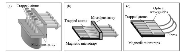
**Fig. 5.** Spatially resolved readout of the internal and external states of atoms (e.g., the state of a qubit) using microlens arrays: (a) Integration of two spherical microlens arrays creates a combined system of dipole traps and efficient detection optics. (b) Integration of a microlens array (for readout) with microfabricated magnetic or electrostatic trapping structures. (c) Optical waveguides and fibres can also be integrated on the substrate.
