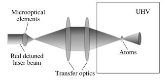
**Fig. 1.** Experimental setup. The light of an incoming red detuned laser beam is focused by a microoptical component and the focal plane is imaged into the vacuum chamber (UHV). Atoms are first collected in a MOT and then trapped in the refocused light field.
