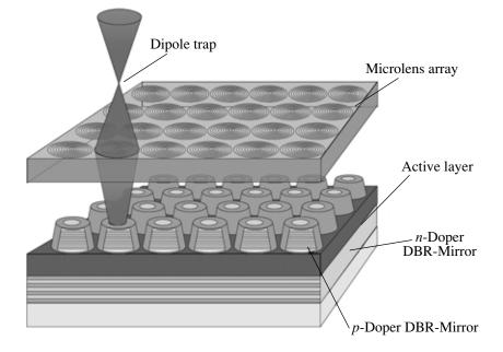
**Fig. 6.** Integration of microoptical components and laser sources. An array of vertical cavity surface emitting lasers (VCSELs) illuminates a microlens array with matched lens separation. Each trap of the resulting two-dimensional array of dipole traps can be individually switched on and off because the individual VCSELs are selectively addressable.
