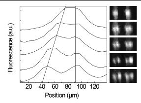
FIG. 6. (Left) Cross sections through pairs of dipole traps as in Fig. 5 (rotated by 90°) for different separations between the traps ranging from 18 to 45  $\mu$ m. (Right) Image sections showing two pairs of traps with decreasing separation from bottom to top corresponding to the cross sections at left.
