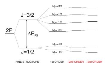
FIG. 1. (Color online) Level scheme of the  $2^2P_J$  states of boronlike argon  $Ar^{13+}$  in an external magnetic field with higher-order contributions to the Zeeman effect (not true to scale).
