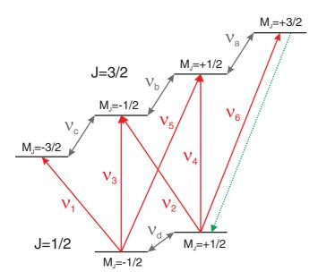
FIG. 2. (Color online) Spectroscopy of the  $2^2P_{1/2}$ - $2^2P_{3/2}$  fine-structure transition, as in a boronlike argon ion  $Ar^{13+}$ , with Zeeman effect. The level scheme (not true to scale) and all magnetic dipole transitions are shown. Solid arrows indicate excitation by laser photons, while dotted arrows are spontaneous decays. Gray double arrows represent microwave transitions.
