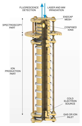
FIG. 7. (Color online) Schematic drawing of the trap. A cut has been applied for presentation of the trap interior.
