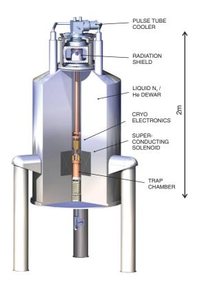
FIG. 6. (Color online) Schematic drawing of the setup. The superconducting magnet has been cut to allow a view of the trap and related components inside the room-temperature bore.
