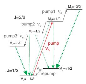
FIG. 4. (Color online) Pump spectroscopy in the Zeeman-split fine-structure doublet. Solid arrows indicate the saturated pumping laser photons, while dotted arrows are spontaneous decays. Projection-conserving decays of the states  $|3/2,+1/2\rangle$  and  $|3/2,-1/2\rangle$  are preferred. Gray arrows represent microwave-stimulated transitions.
