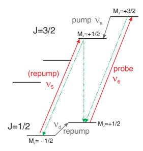
FIG. 3. (Color online) Probe spectroscopy in the Zeeman-split fine-structure doublet. Solid arrows indicate the saturated probing and, optionally, pumping laser photons, while dotted arrows are spontaneous decays. Gray arrows represent microwave-stimulated transitions.
