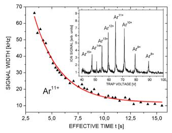
**Figure 8.** Spectral width of the detected signal of  $Ar^{11+}$  ions as a function of the effective cooling time. The curve is an exponential decay fitted to the data. Inset: spectrum of confined argon-ion charge states as produced by the internal ion source.
