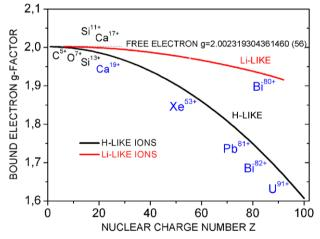
**Figure 2.** Theory predictions of the magnetic moment (*g*-factor) of the electron bound in hydrogen-like and lithium-like ions as a function of nuclear-charge number *Z*. The indicated ions with charge states below Z = 20 have been measured so far; the others are prominent candidate ions. Note that on this scale, experiment and theory values are indistinguishable and experimental uncertainties vanish within the line thickness.
