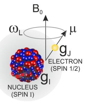
**Figure 1.** Cartoon of a hydrogen-like ion and the quantities involved: a single electron is bound to an atomic nucleus. The precession of the electron spin around the external magnetic field  $B_0$  of the Penning trap at the Larmor frequency  $\omega_L$  yields the magnetic moment  $\mu$  and hence the electronic g-factor  $g_I$ .
