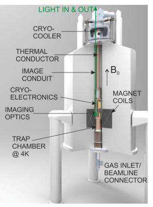
**Figure 5.** Cutout of the setup consisting of a cryogenic Penning trap arrangement in the center of a superconducting magnet. The light (excitation laser and fluorescence signal) is guided to and from the trap via an image conduit.
