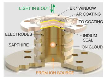
**Figure 6.** Cutout of the dedicated spectroscopy trap, which is a half-open cylindrical Penning trap with a window endcap that has a conductive coating on the inside. The excitation laser beam enters from above, ions from below. Fluorescence is collected through the window.
