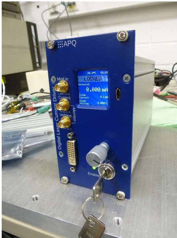
Ultra-stable Digital Laser Current Driver
