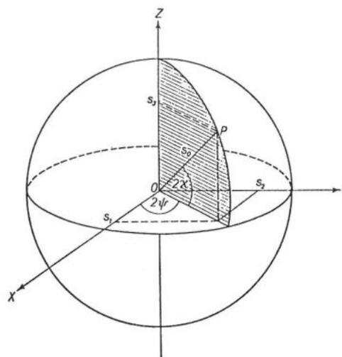
Figure 2 The Poincaré representation of polarized light on a sphere.
