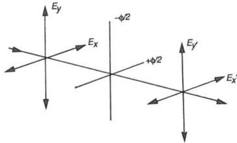
Figure 4 Propagation of a polarized beam through a retarder.
