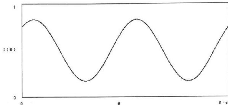
Figure 7 Intensity plot of an elliptically polarized beam for  $\alpha = \pi/6$  and  $\delta = \pi/3$ .
