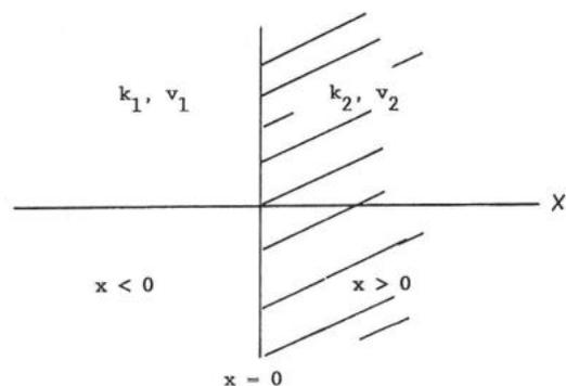
**Figure 4** Reflection and transmission of a wave at the interface between two media.
