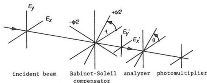
**Figure 5** The measurement of the ellipticity and orientation of an elliptically polarized beam using a compensator and a photodetector.
