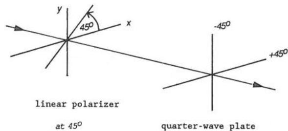
**Figure 2** Construction of a circular polarizer using a linear polarizer and a quarter-wave plate.
