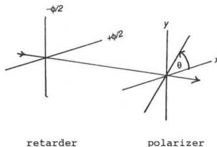
Figure 3 Measurement of the Stokes polarization parameters.
