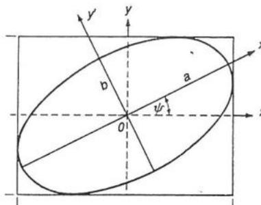
Figure 3 The rotated polarization ellipse.
