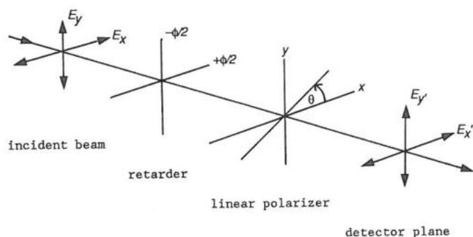
Figure 1 Classical measurement of the Stokes parameters.
