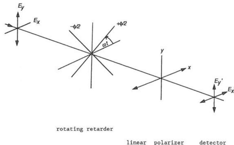
**Figure 4** Measurement of the Stokes parameters using a rotating quarter-wave retarder and a linear polarizer.
