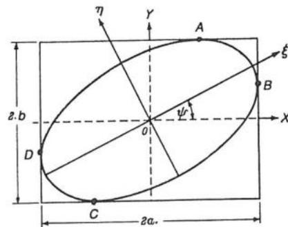
Figure 2 An elliptically polarized wave and the polarization ellipse.
