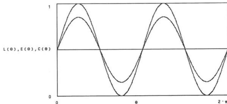
Figure 8 Plot of the intensity for a linearly polarized beam, an elliptically polarized beam, and a circularly polarized beam.
