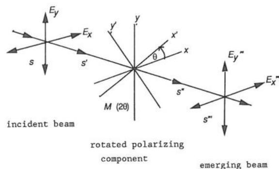
**Figure 6** Derivation of the Mueller matrix for rotated polarizing components.
