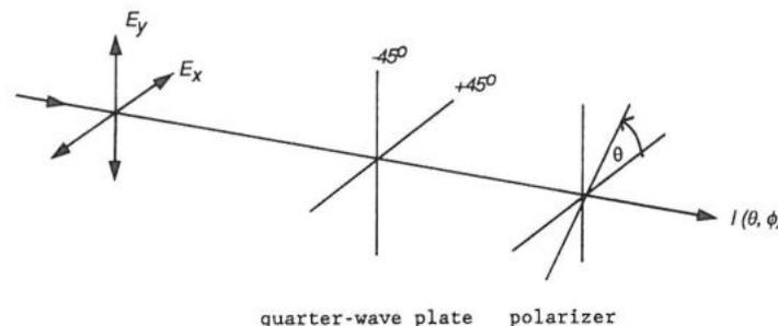
Figure 6 Experimental configuration to determine the state of polarization of an optical beam.
