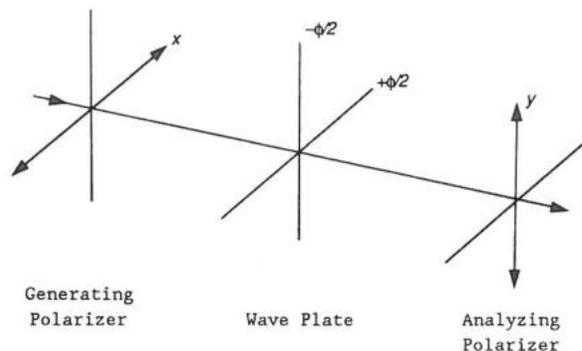
Figure 2 Crossed polarizer method to measure the phase of a wave plate.
