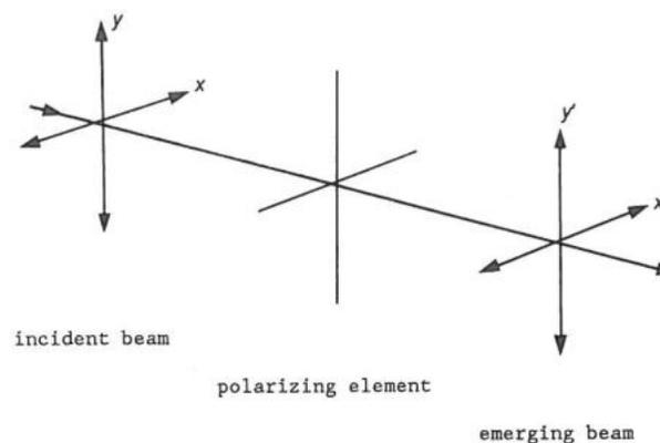
**Figure 1** Interaction of a polarized beam with a polarizing element.
