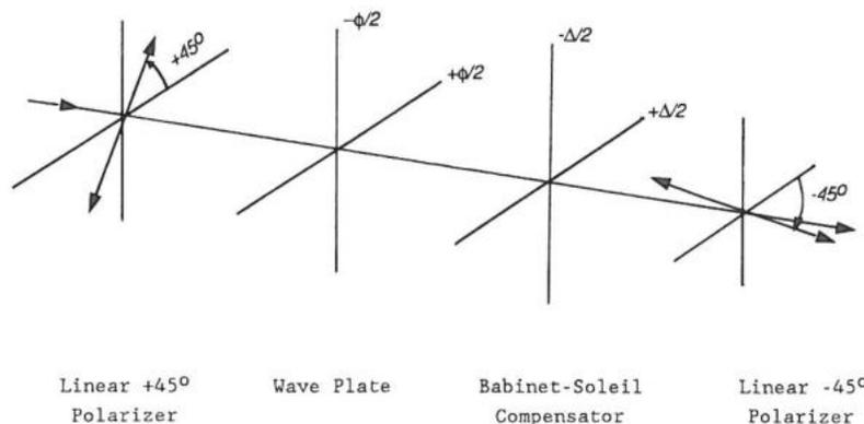
Figure 3 Measurement of the phase shift of a wave plate using a Babinet-Soleil compensator.
