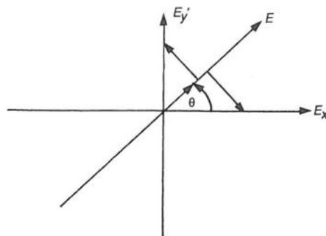
Figure 4 Resolution of the optical field components by a polarizer.
