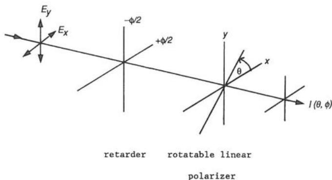
Figure 3 Null intensity measurement of the Stokes parameters.
