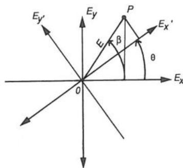
Figure 5 Rotation of the optical field components by a rotator.
