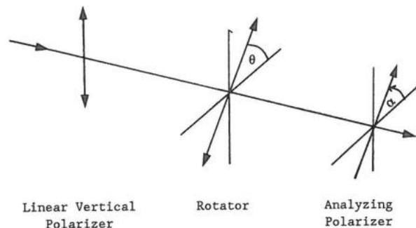
Figure 4 Measurement of the rotation angle  $\theta$  of a rotator.
