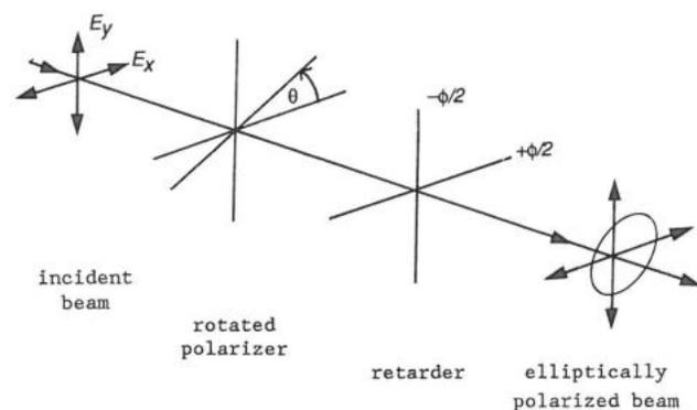
Figure 7 The generation of elliptically polarized light.
