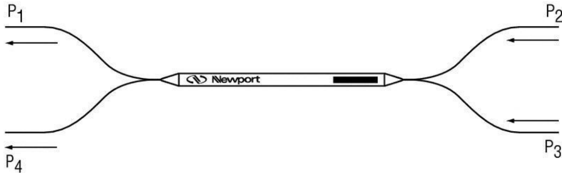
Figure 3. A 1x2 or a 2x2 coupler.
