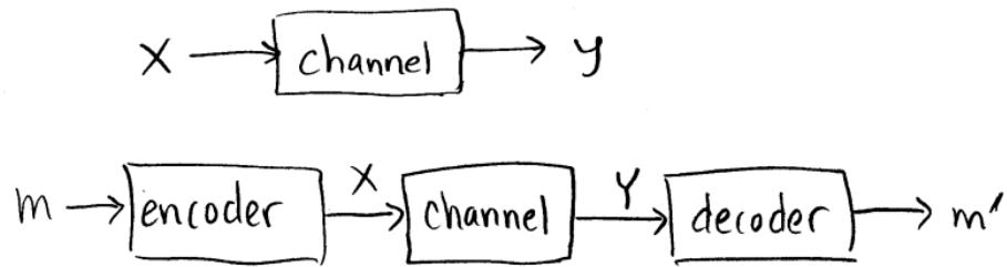
Use an encoder and decoder to transmit messages  $m$  reliably.
