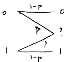
$$\text{try } q = \frac{1}{2} \quad H(X) = 1 \quad H(Y) = -(1-p) \log \frac{1-p}{2} - p \log p = h_2(p) + (1-p)$$
