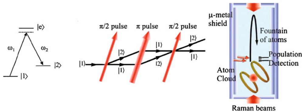
**Fig. 1** Atom interferometry accelerometer; from left to right: Raman transition between the hyperfine levels of an alkali atom; Mach-Zender atom interferometry scheme implemented with three Raman pulses ( $\pi/2 - \pi - \pi/2$ ): the direction of the red arrows represent the effective momentum transferred in the stim-
