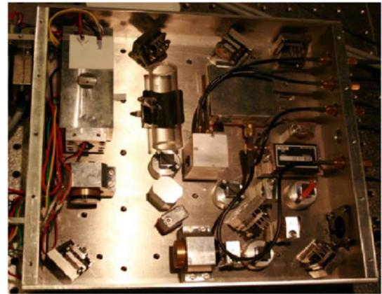
**Fig. 7** *Left*: scheme of the modular laser system; *right*: a picture of the master laser module
