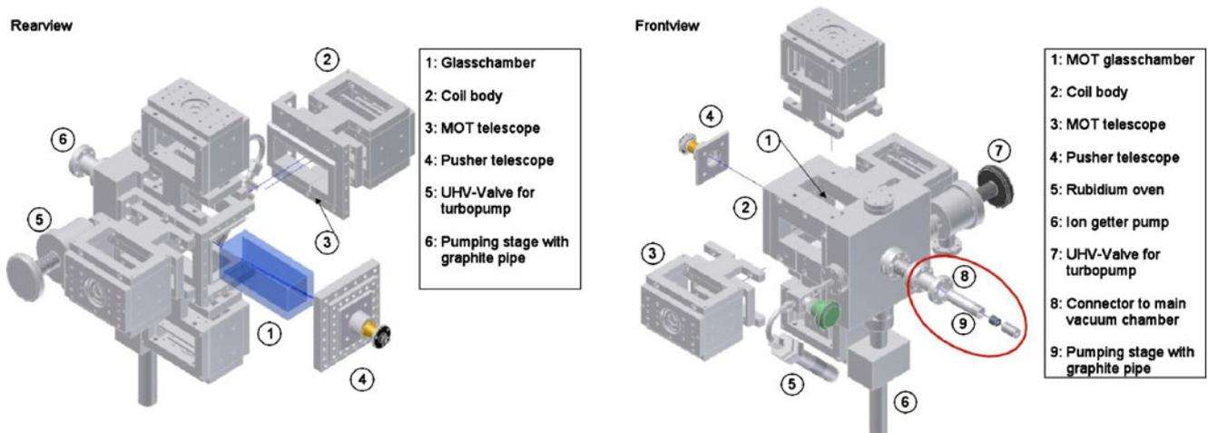
**Fig. 6** 3D views of the mechanical structure of the 2D-MOT system
