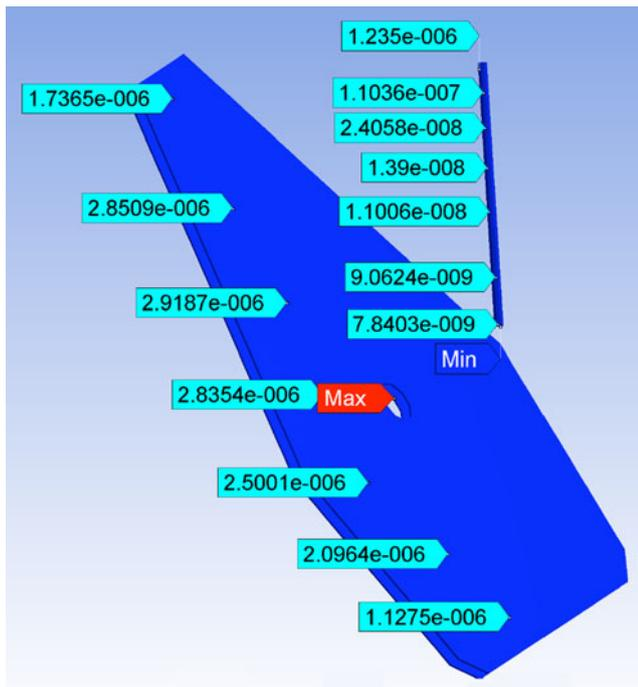
**Fig. 5** Numerical calculation of residual magnetic field inside the capsule; the labels indicate the amplitude of magnetic field (in Tesla) on different points of the diagonal  $\mu$ -metal plane and along the atomic trajectory (from the center of the chamber to the upper edge of the tube) when an external bias field of 50  $\mu$ T is applied along the vertical axis
