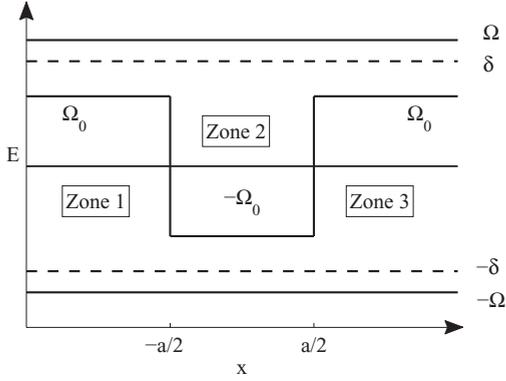
FIG. 1. Schematic drawing of spatial variation of frequencies in an optical 0- $\pi$ -0 Josephson junction for cold atoms: the Rabi frequency  $\Omega_0(x)$ , the detuning  $\delta$ , and the generalized Rabi frequencies  $\pm\Omega$ , which are constant throughout the system. The junction's domains are localized at  $\pm a/2$  (all variables dimensionless).
