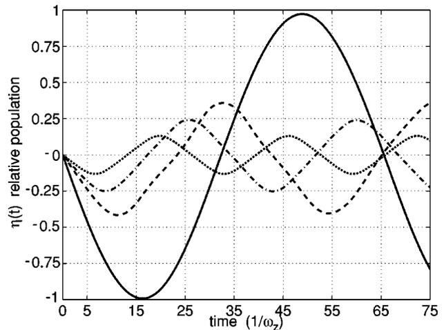
FIG. 3. Plot showing that the effect of the displacement  $z_0$  on the system is to suppress the amplitude of oscillation. The four curves represent increasing values of  $z_0$ : 0 (solid), 0.1 (dashed), 0.2 (dash-dotted), and 0.5 (dotted). In each case, the detuning  $\delta$  is chosen so that the system is initially being driven resonantly, and the initial phase is  $\phi(0) = \pi/2$ .
