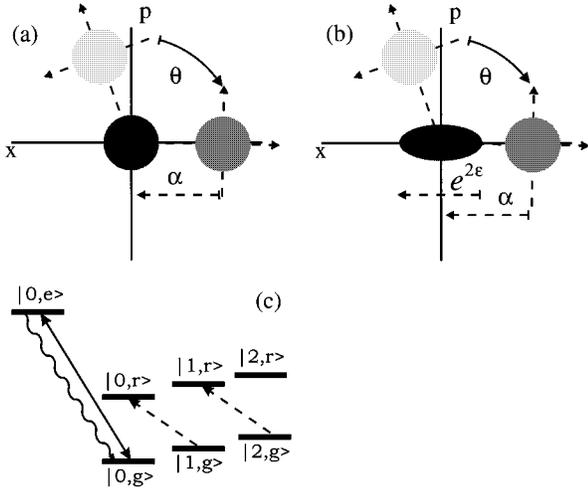
FIG. 1. Phase-space representation of the operations (phase shifting, displacement, and squeezing) required to measure (a) the  $Q(\alpha)$  function and (b) the quadrature distribution; (c) level scheme and laser configuration for the detection of the trap ground-state population.
