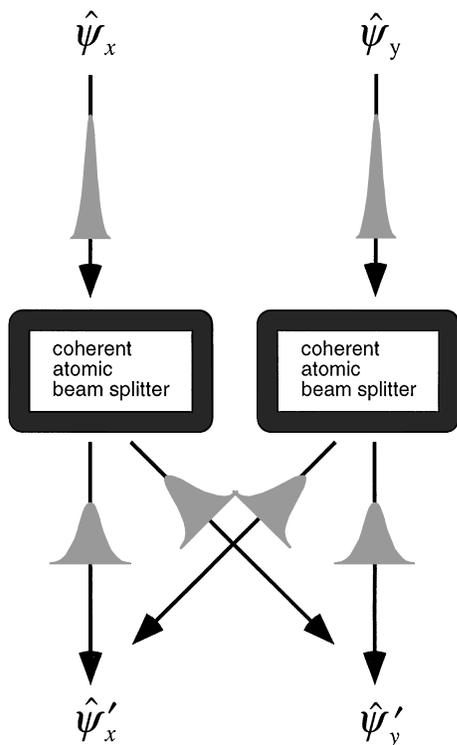
FIG. 1. Two orthogonal position modes  $|x\rangle, |y\rangle$  of a massive field  $\hat{\psi}$  are selected by a double slit. As the particles propagate downstream, they are coherently superimposed by atomic beam splitters and collected by two detectors.
