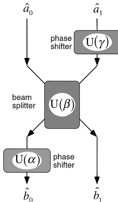
FIG. 2. Setup of an optical beam splitter. Two optical modes  $a_0$  and  $a_1$  of orthogonal propagation direction or polarization are phase shifted  $[U(\gamma), U(\alpha)]$  and mixed coherently in a general nonbalanced beam-splitter device  $[U(\beta)]$ .
