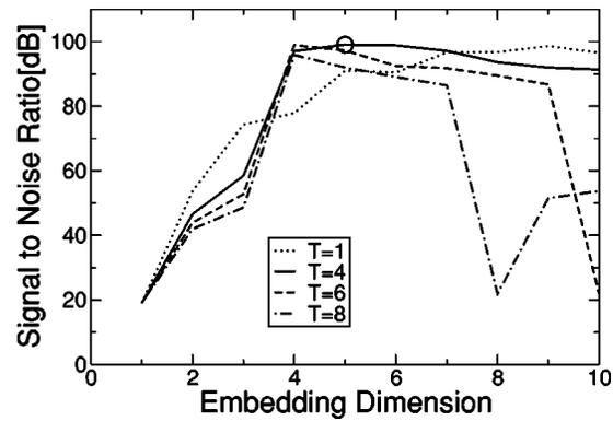
FIG. 7. Signal-to-noise ratio as a function of embedding dimension for various values of the time-shift  $T$ . The best approximation of all data points (see circle) is determined for the numerical example of the duffing oscillator.
