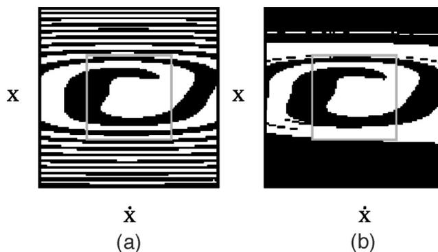
FIG. 2. Basins of attraction of two coexisting attractors of the Duffing oscillator for  $100 \times 100$  initial conditions. (a) Direct calculation via the differential equation. (b) Calculation via the approximated global flow. Black: periodic; white: chaotic. The gray square in the middle shows the region used for the approximation.
