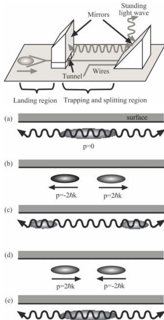
**Figure 8** Schematic drawing of the atom-Michelson-interferometer (not to scale). The dimensions of the chip are  $5\ \text{cm} \times 2\ \text{cm}$ . a–e) Interferometric sequence (see text). Adopted from [63].
