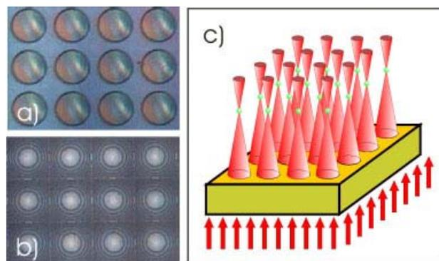
**Figure 5** Illuminating a two-dimensional array of refractive (a) or diffractive (b) micro-lenses with near-resonant laser light gives a two-dimensional array of dipole traps for neutral atoms (c) which can serve as a quantum register for atomic qubits [68].
