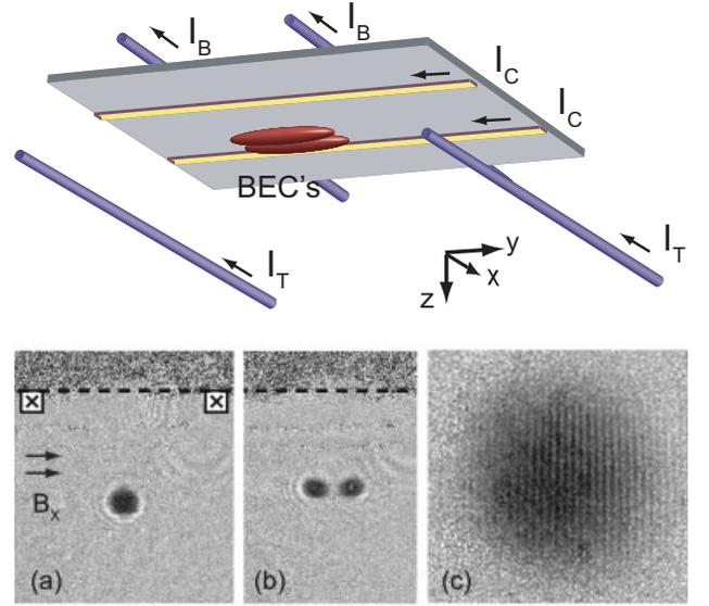
**Figure 10** Schematic diagram of the two-wire beam splitter. A magnetic double-well potential is created by two chip wires with a current  $I_C$  in conjunction with an external magnetic field. Splitting of a condensate for increasing external field and (c) the interference pattern of condensates split to a distance of  $25.8 \mu\text{m}$  as observed after 22 ms free expansion. Adopted from [60].
