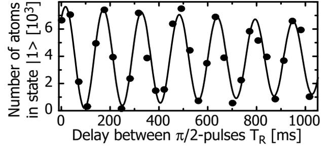
**Figure 4** Ramsey fringes observed for a hyperfine transition of  $87\text{Rb}$  atoms held at a distance of  $d = 9 \mu\text{m}$  from the metallic surface of a chip. The experiment demonstrates a single qubit operation. Adopted from [62].
