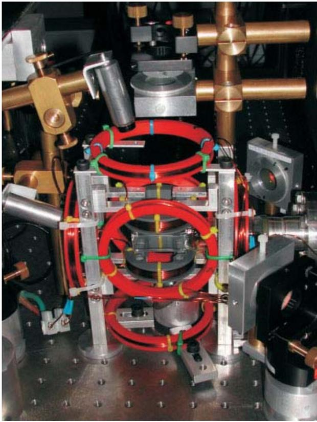
**Figure 2** Typical experimental setup. Alkali atoms are trapped and cooled in a configuration called ‘magneto-optical trap’ inside a glass vacuum cell at the center of a set of coils for magnetic fields. Temperatures in the range of 10 to 100  $\mu\text{K}$  can be achieved. This prepares atomic quantum systems for further experiments on quantum information processing and matter wave interferometry [68].
