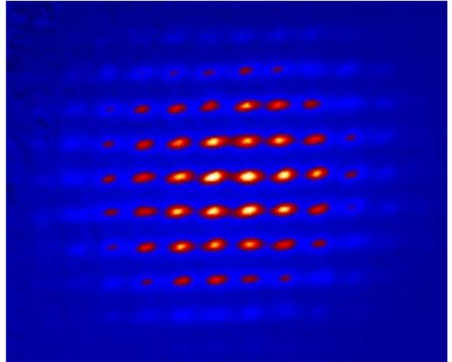
**Figure 1** A two-dimensional set of atom ensembles in optical dipole traps based on arrays of micro-lenses can serve as a qubit register. Individual traps in this fluorescence image have a lateral separation of  $125\ \mu\text{m}$  [68].
