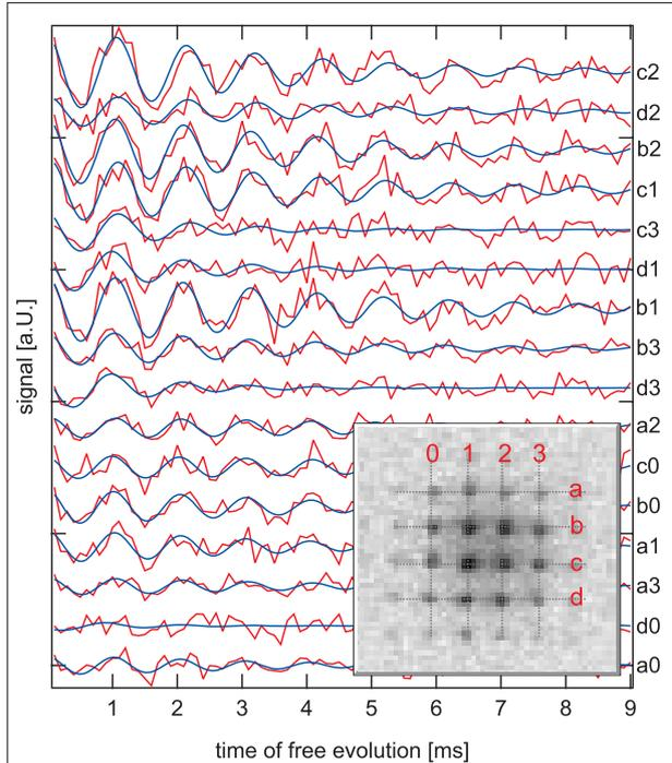
**Figure 6** Simultaneous Ramsey measurements in 16 different dipole traps. The associated position of the traps is shown in the inset. The inset is a fluorescence image of the atoms trapped in the two-dimensional trap array Adopted from [39].
