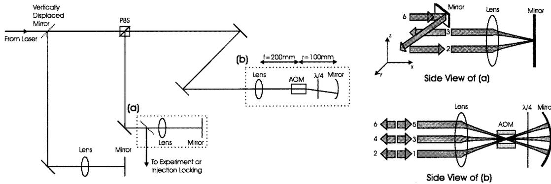
FIG. 1. Optical configuration for frequency shifting of a laser field by 1.518 GHz using a single low frequency acousto-optic frequency shifter (AOM). The AOM is operated at 253 MHz in sixtuple pass (i.e., three double passes). We have obtained an overall efficiency of up to 24%.
